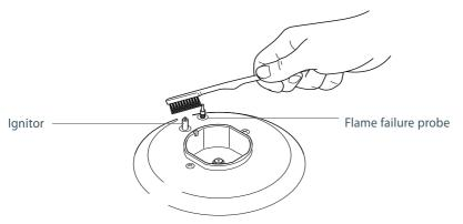
Figure 20 Cleaning the probe and ignitor
